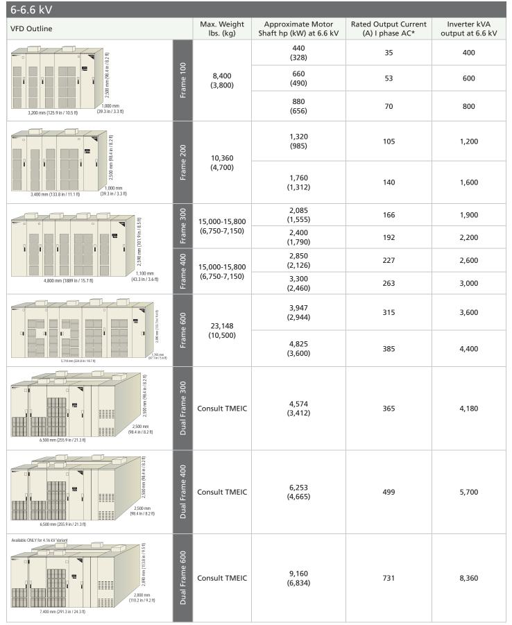
\* 1: 110% OL for 60 sec. Panel heights include cooling fans. VFD capable of 80% regeneration at nominal voltage at unity power factor. Frame designation indicates power cell rating for replacement parts and other purposes.
