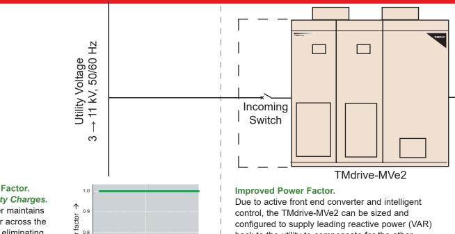
configured to supply leading reactive power (VAR back to the utility to compensate for the other lagging loads on the same bus, or at the point of common coupling, thereby significantly improving the power factor as seen by the utility.
