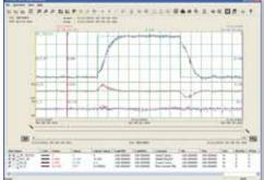
High speed data is automatically captured and saved in the event of a drive fault. Users can capture high speed data based on their own trigger conditions or perform high resolution real-time trending.
