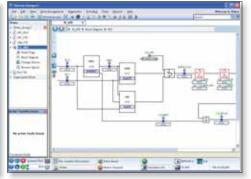
Live block diagrams provide a realtime graphical view of drive functions. Functions can be configured directly from the graphical view.
